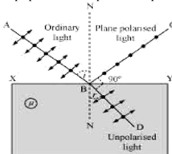
The parallel component of light is converted into perpendicular component and gets reflected from the interface. The parallel component of light is continues to vibrate and get refracted or transmitted. As a result of which the reflected component is polarised.
