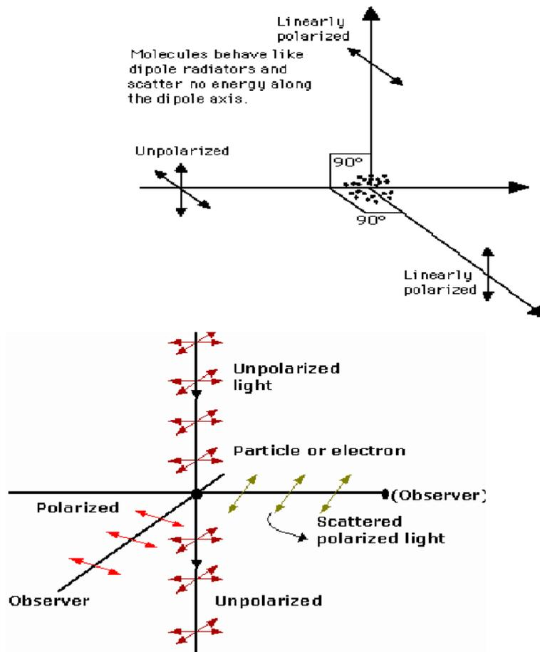
To explain the phenomenon of scattering, let us consider a beam of unpolarised light along z-axis on a scatter at origin. As light waves are transverse in nature in all possible direction of vibration of unpolarised light is confined to X-Y plane. When we look along X-axis we can see the vibrations which are parallel to Y-axis. Similarly, when we look along Y-axis the vibration along X-axis can be seen. Hence, the light can be scattered perpendicular to incident light is always plane polarized.
