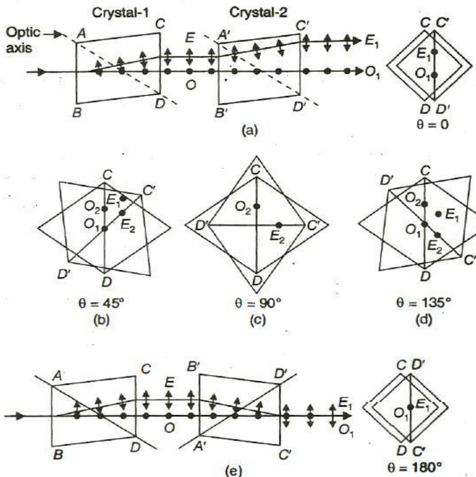
This is how we are able to produce the plane polarised light by the method of double refraction.
