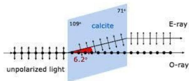
When the light passing through the crystal along the optic axis then at the optic axis the ray splits up into two rays called as ordinary and extraordinary ray which get emerge parallel from the opposite face of the crystal through which are relatively displaced by a distance proportional to the thickness of the crystal. This phenomenon is called as double refraction.
