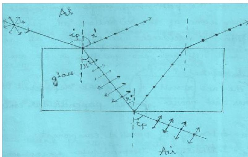
To explain the polarization by refraction, let us consider an ordinary light which is incident upon the upper surface of the glass slab at an polarizing angle  $i_p$  or Brewster's angle  $\theta_B$ , so that the reflected light is completely polarized while the rest is refracted and partially polarized. The refracted light is incident at the lower face at an angle "r".
