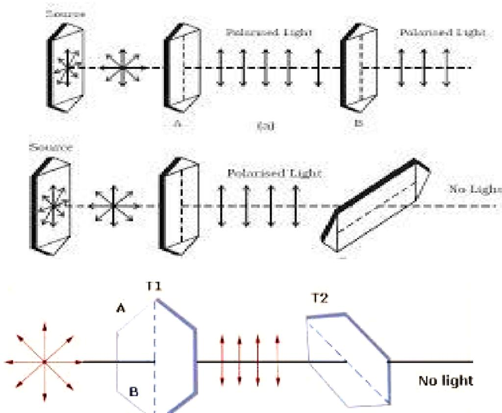
The intensity is maximum when the axis of  $T_2$  is parallel to that of  $T_1$  and minimum when they are at right angle. This shows that the light emerging from  $T_1$  is not symmetrical about the direction of propagation of light but its vibrations are confined only to a single line in a plane perpendicular to the direction of propagation, such light is called as polarised light.
