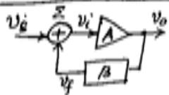
part of output signal (voltage or current), is in phase (180°) with the input signal and hence enhances/increases it.
