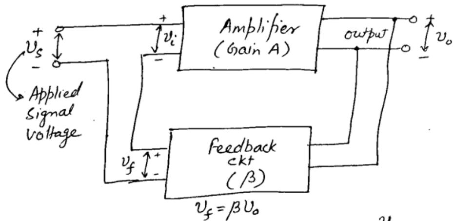
$$A = \text{Gain of the Amplifier ckt} = \frac{V_o}{V_i}$$
